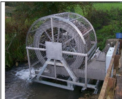
Modern water wheel that generates electricity
